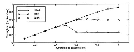
Figure 4. Throughput of LEAP versus the aggregate normalized network offered load.
