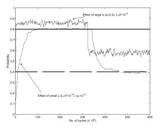
Figure 3. Effects of a small value of the learning rate L and of a large value of parameter a on PLR-P LA convergence
