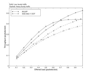
Figure 5. Throughput of AHLAP and IEEE 802.11 DCF, for low and high grade bursty traffic, versus the aggregate normalized offered load to the network.
