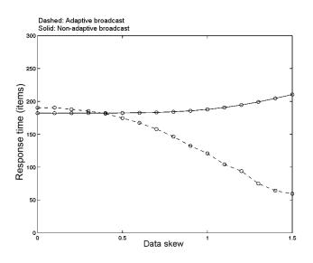
Figure 6: Performance gains of the method of [19] due to the incorporation of adaptivity.
